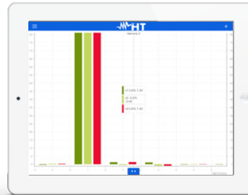
Current and voltage harmonics
