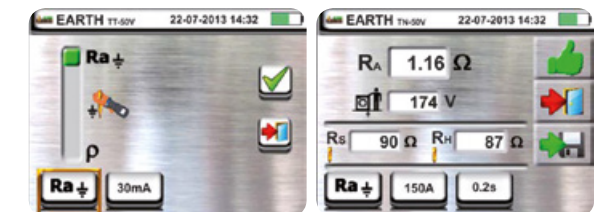
Earth resistance measurement by Volt-ampere method
