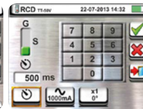
Setting of RCD delayed time
