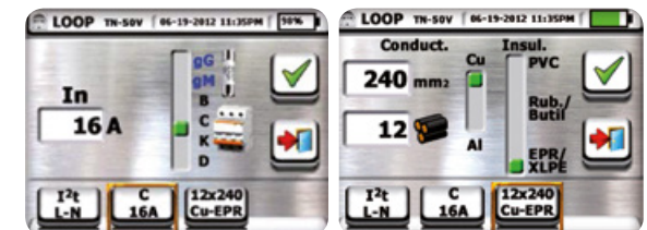
Setting of MCB/fuse type and rated current
