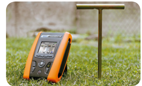
Earth resistance measurement by Volt-ampere method
