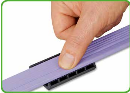
Insert flat cable into base (observe coding!).
