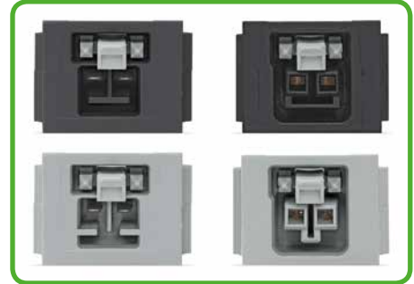
B-coded connectors (shown in gray) not only differ in color, but also in their design, making them incompatible with other coded connectors.
