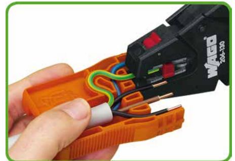
Strip conductor ends 9 mm (see marking).
