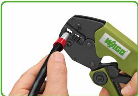
Insert ferruled conductor into crimping station.
