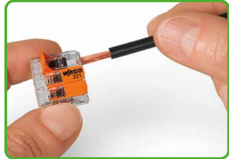
Termination: Open clamping unit using the lever and insert conductor.
