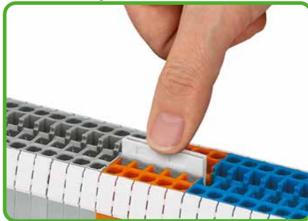
Push jumper bars down firmly until fully inserted. When using multi-pole bars, push alternately on right and then left side, successively until installed.
