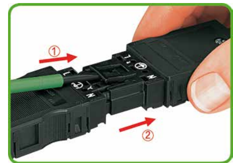
Locking lever, tool operated: 1.) Unlatch locking lever. 2.) Pull apart the connectors. (Example shows 3-pole connectors)
