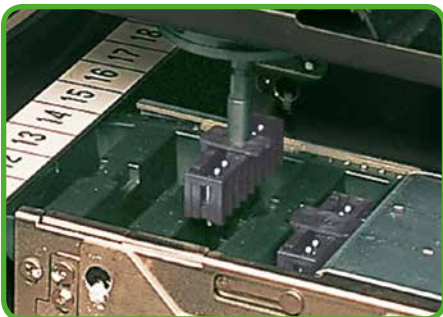
THR male headers for reflow soldering in SMT production.
