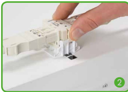
2 Slide the connector toward the square recesses until it stops.
