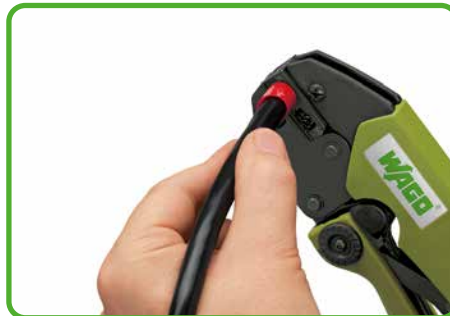
Squeeze handles until ratchet mechanism is released.
