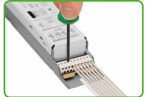
Removing conductor via 1.0 mm Ø disconnection tool.
