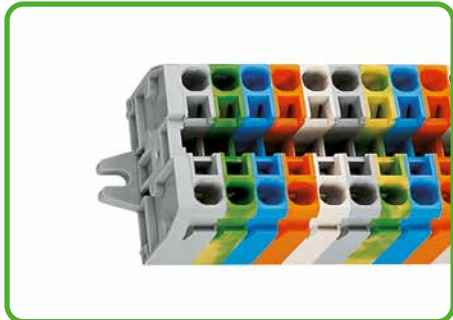
Terminal strips with fixing flanges M3 or M4, for screw or mounting types, mounting holes 3.2 mm Ø, flange M3 4.2 mm Ø, flange M4
