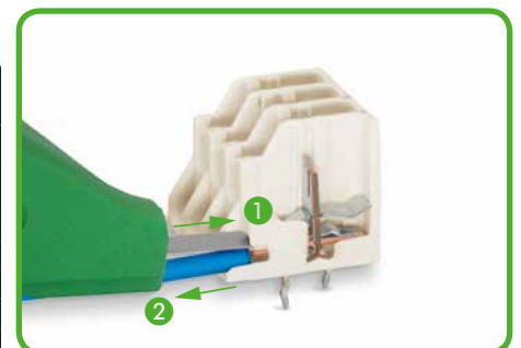
Conductor removal – "251 mini" PUSH WIRE®: Twist conductor and pull out, or fully insert 206-830 disconnection tool over the conductor and pull it out. FIT CLAMP® (IDC): Pull up vertically on conductor to remove it (10 x reconnection possible when used properly. Before re-using, cut off old contact point from conductor)
