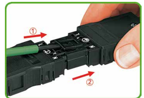
Locking lever, tool operated: 1.) Unlatch locking lever. 2.) Pull apart the connectors.
