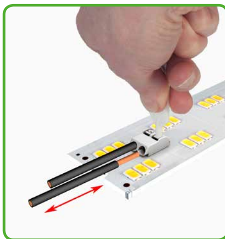
Inserting/removing fine-stranded conductors by lightly pressing on push-button.
