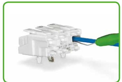
Conductor removal: Slide disconnection tool beneath the conductor and pull conductor out.
