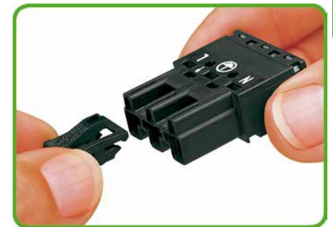
Snap on locking lever. Observe direction! (Example shows 3-pole plug)
