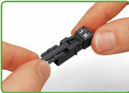
All connectors (snap-in versions, distribution connectors) for fixed installations are factory-equipped with locking levers to ensure plugs and sockets are securely locked. Additional locking levers are only required for "flying leads" (plug/socket).
