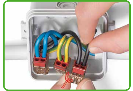
Removal: Hold conductor to be removed and twist alternately left and right while pulling the connector.
