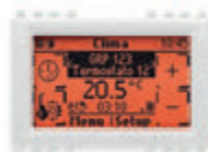
21509.B For control and configuration, touch display, temperature sensor input, for DIN rail (60715 TH35) or mounting installation - 3 modules. Depth: 37 mm
