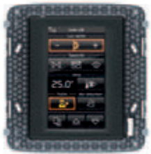
■ 20848.1 Color touch screen, 4,3", for the control, 1 temperature sensor input, with built-in mounting frame for installation in 8-module mounting box. Depth: 39,9 mm
