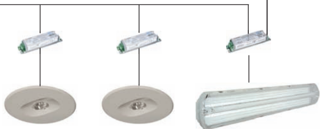
Emergency luminaires in maintained mode
