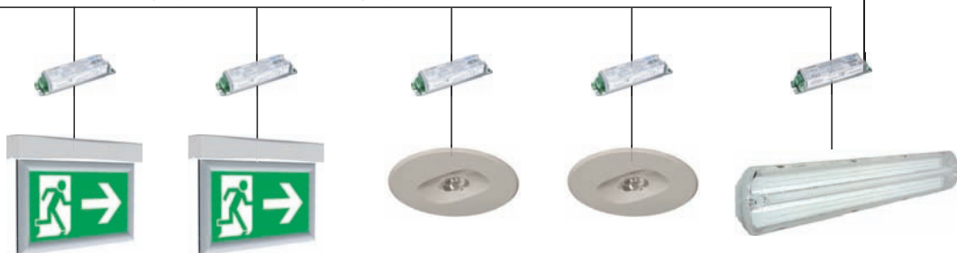
Emergency luminaires in non-maintained mode
