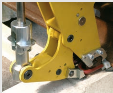
Extraction and insertion of Pandrol "Fast clips".
